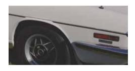
Bottom of thick stripe is 16mm above the rear badge at highest point. Cut is in the thick stripe only over the wheel arch at a radius of 30mm from the wheel arch. The thin top line continues straight across the top of the wheel arch good adhesion.
